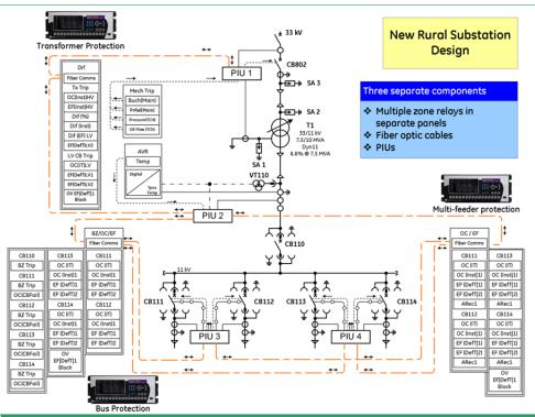
Figure 2: New small rural substation design
